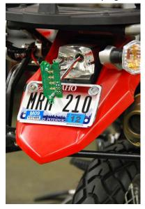
4. Align the mounting tabs with the screw bosses.
