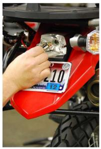
3. Insert the LED module plug into the socket.
