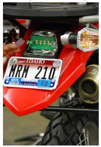
6. Replace the rear cover and screw it back in place, making sure that the screws pass through the slots in the mounting tabs.
