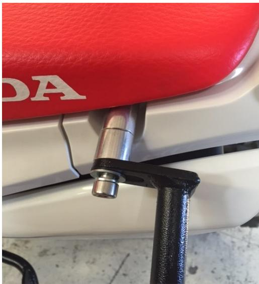
Figure 2: Center mounting point on SU Rack
