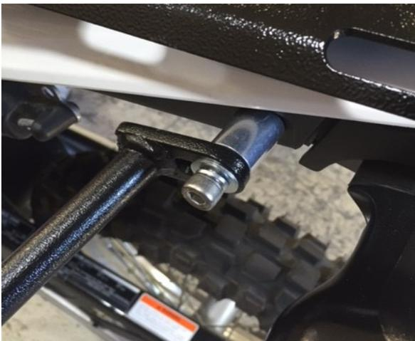
*Figure 4: rear mounting point on SU Rack*
