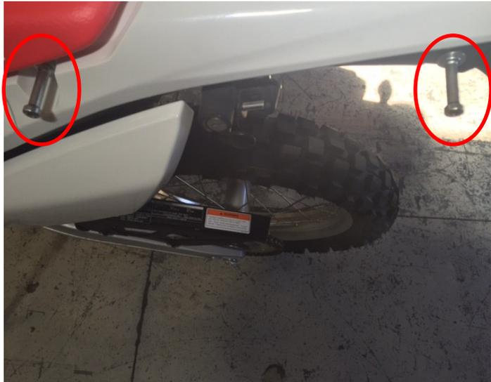
Figure 1: Tie down points circled in picture above.
